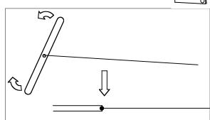
The etched mounting is angled to ensure the DA valve is vertical once fitted. Position the valves about 10mm from the brake pivot bar (towards the end of the floor). If required, a short length of soft copper wire can be fixed to the top of the valve and into the bottom face of the brake cylinders (see photos on our CD).
