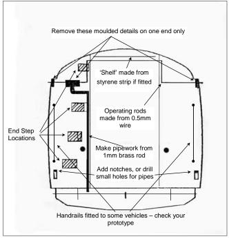
evidence of the positions of the steps remains when the steps themselves have been removed. You can simplify the preparation of the ends by simply leaving the small rectangular pads in place on the end mouldings. Alternatively, flush ends can be modelled by carefully paring off the moulded pads and sanding the areas smooth. Also some catering cars had short vertical handrails on the ends. Attend to these points now...
