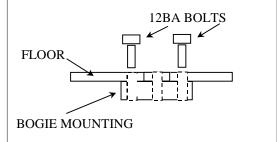
27) To make a much stronger job of fixing the bogie pivots in place, you might consider a 'belt and braces' approach by adding a mechanical fixing to the
